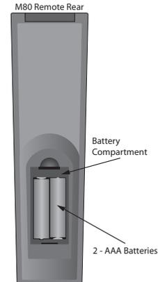
**Diagram 77** Installing M80 Remote Control Batteries
