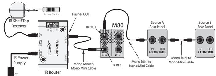
**Diagram 22** IR IN/OUT Connections with IR Control Inputs
