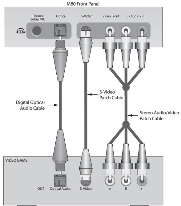
**Diagram 26** Front Panel A/V Connections
