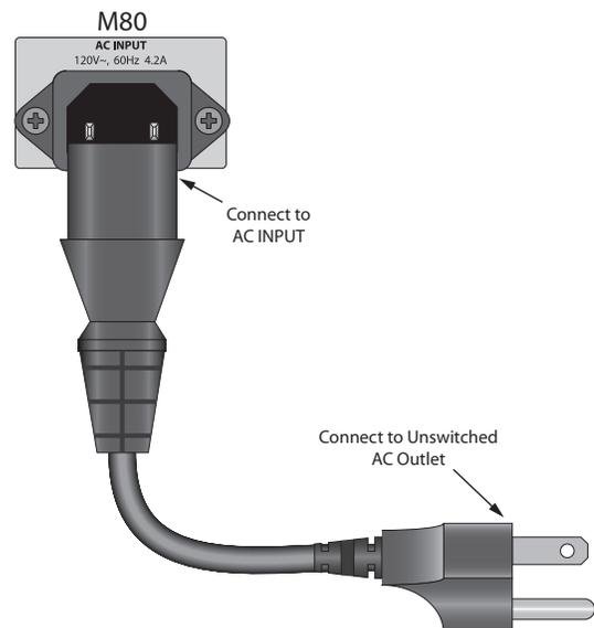
**Diagram 25** AC Power Cord Connections
