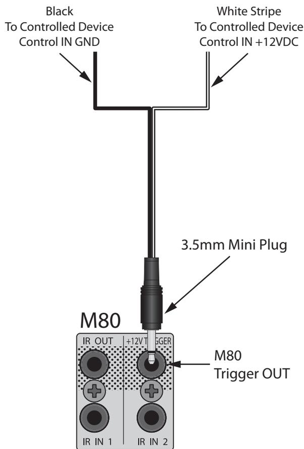
**Diagram 20** Trigger Out Connections
